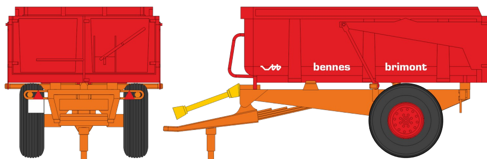
CB-222 : Remorque BRIMONT simple essieu châssis orange BRIMONT single-axle trailer with orange chassis
